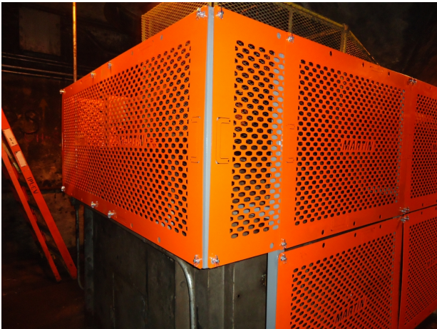
Martin Engineering's guarding increases safety by restricting access to moving parts and pinch points.
