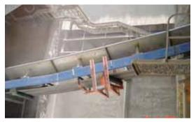
The Martin® Air Supported Conveyor installed at Cementos Progreso was engineered with a vertical curve in the center third of the conveyor's 156-foot (47.7-m) length.
