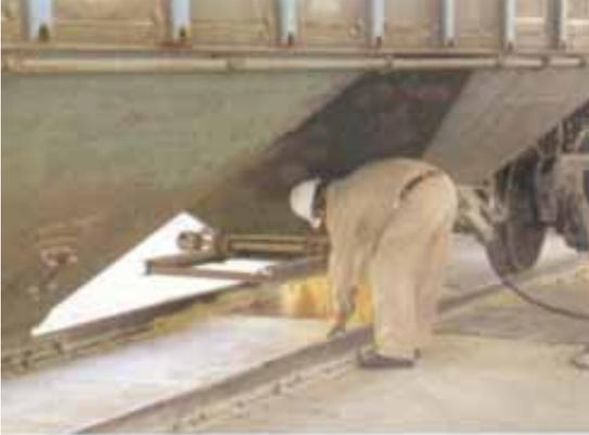
*The heavy pneumatic vibrators used to assist the unloading of railroad hopper cars at the cement plant were noisy and risked back injuries.*
