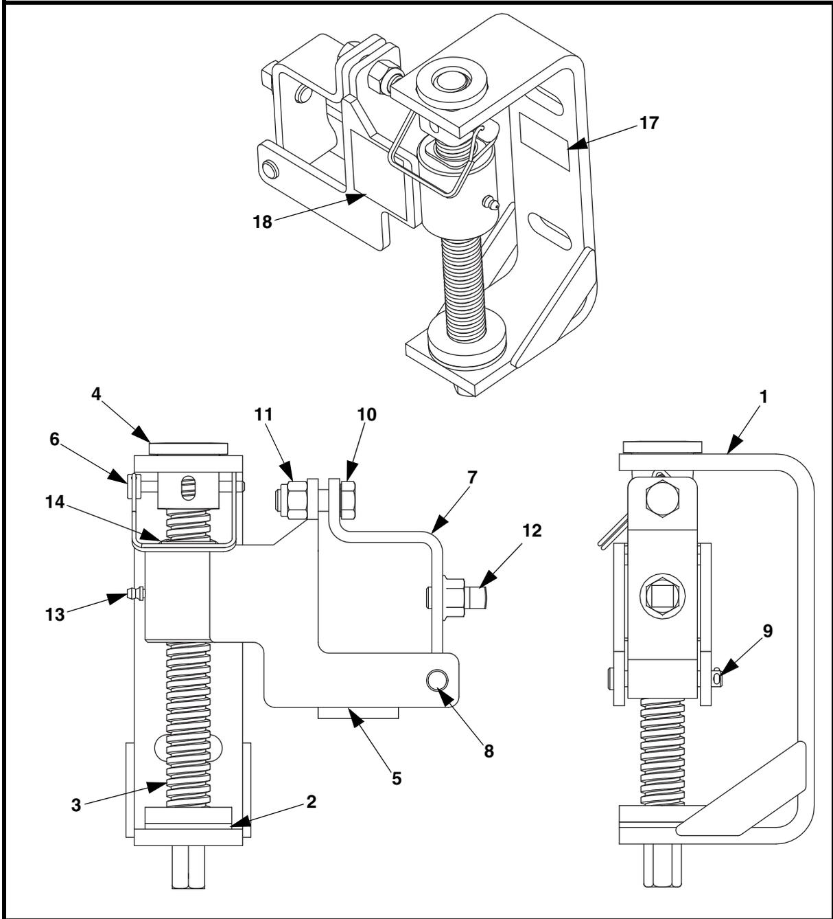
Figure 1. Martin® SQC2S™ Square Mainframe Tensioner Assembly, P/N 38664
