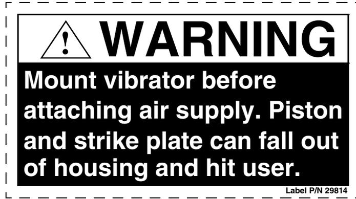
Figure 13. Piston Vibrator Warning Label, P/N 29814
