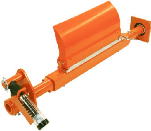
The [Martin® QC1™ Cleaner HD Max](#) tackles the tough jobs. Designed for rugged conditions, this sturdy cleaner features a one-pin blade change, making replacement of a worn blade a simple procedure.
