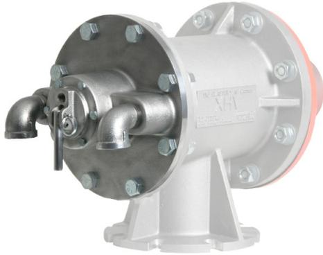
The [Martin® Tornado Retrofit Valve](#) produces better material flow with greater force, faster cycling, and improved safety. The Martin® Tornado Air Cannon fires when the exhaust valve opens in response to a positive surge of air sent by a tripped solenoid valve. This positive-acting valve amplifies the discharge force, up to 20% more force than a standard Martin® XHV Air Cannon of the same size.
