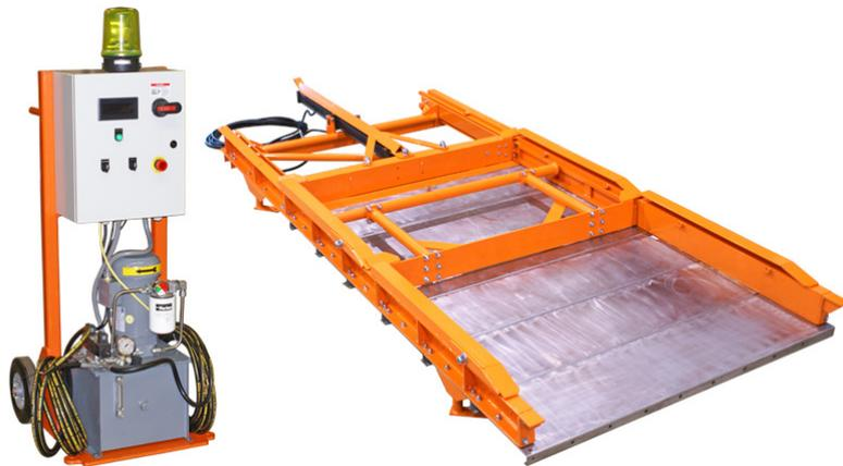
The [Martin® Carryback Capture System](#) is designed to return carryback from secondary and tertiary cleaners to the main cargo stream. Carryback from secondary and tertiary cleaners falls into the collecting trough and is pushed back into the material flow by steel cleaning blades.
