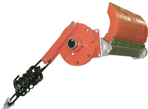
The [Martin® ZHD Cleaner](#) use advanced engineering and superior understanding of material performance to provide effective belt cleaning and compensate for severe-duty conditions and abrasive wear. Installed on the face of the head pulley, the Martin® ZHD Cleaner flexes under tension to provide effective cleaning and overcome uneven wear.
