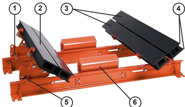
Installed under the skirtboard of a transfer point, [Martin® Slider Cradles](#) support the edges of the belt to eliminate sag. These cradles prevent transfer point spillage by stabilizing the belt's path and allow the effective sealing of the belt edge. Cradles are available with high-performance UHMW or Stainless Steel Bars to match application requirements.
