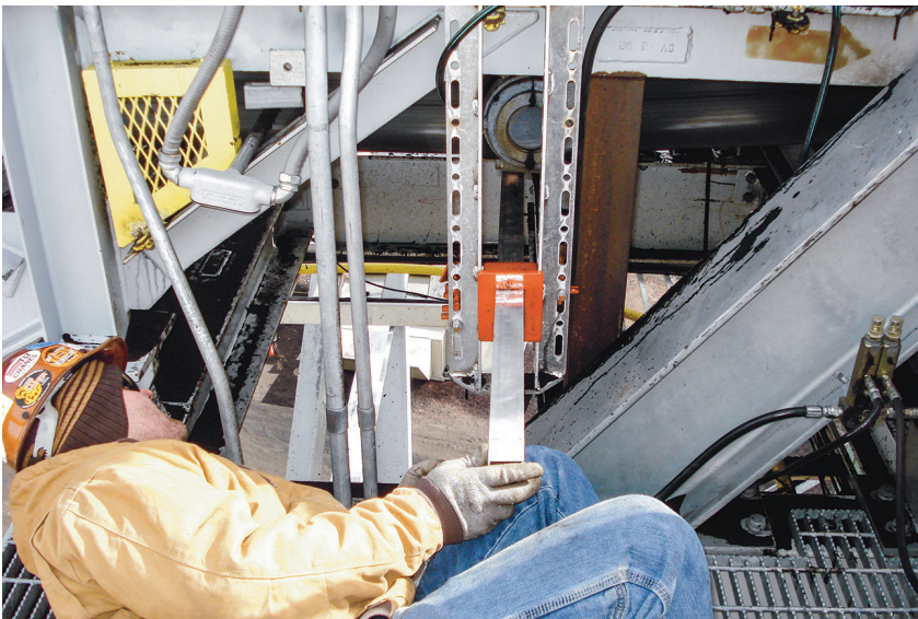
The Martin Conveyor Belt Carryback Gauge is a patented tool designed for estimating the amount of carryback on the return side of a conveyor belt.
