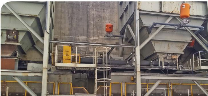
**The innovative solution includes two 100 litre Martin® XHV Air Cannons at the back of the bin.**
